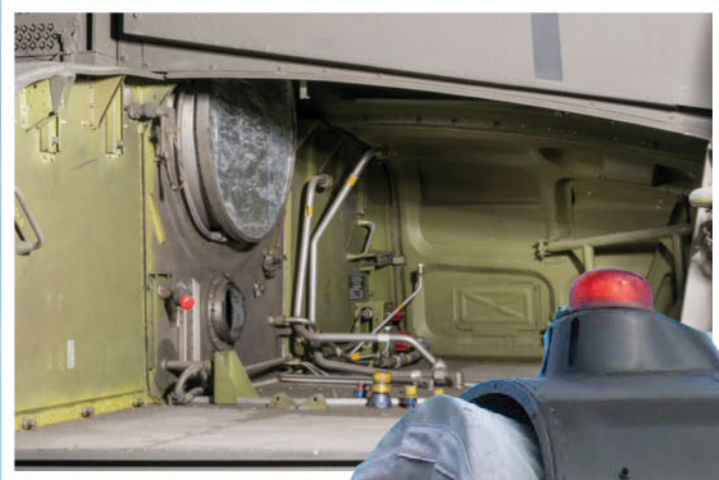
Above: This small empty space would have housed the turbine engine, enabling a greater amount of cargo and passenger space
